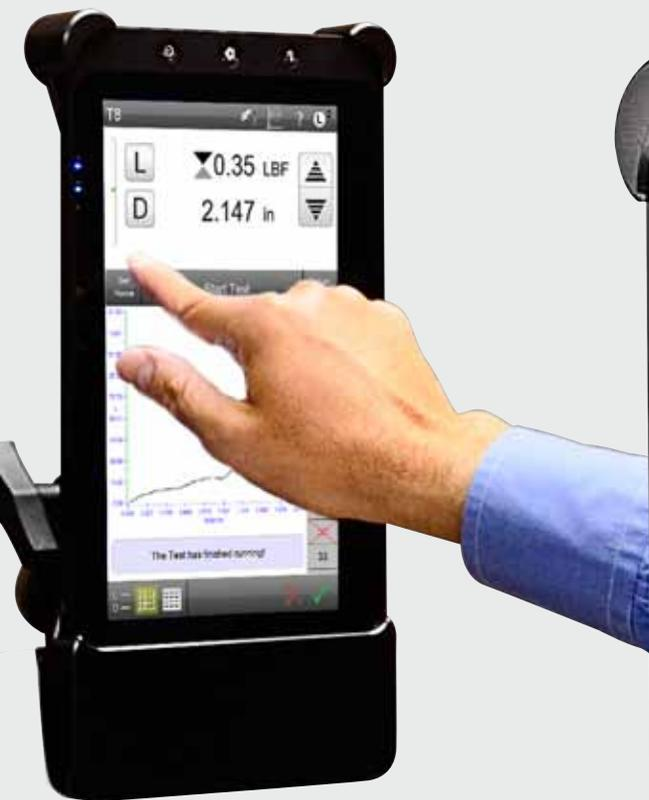
Our L2 controller is a tablet computer featuring a 10-inch (254mm) color, touchscreen display. The controller is both WiFi® and Bluetooth® compatible with two USB 2.0 ports. Exporting your results to a network device is simple, seamless and transparent.
